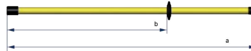
Indoor application earthing stick
